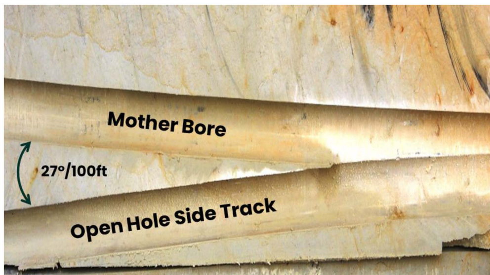
Figure 9—Cut view of a sandstone block showing an open hole sidetrack with an RSM2
