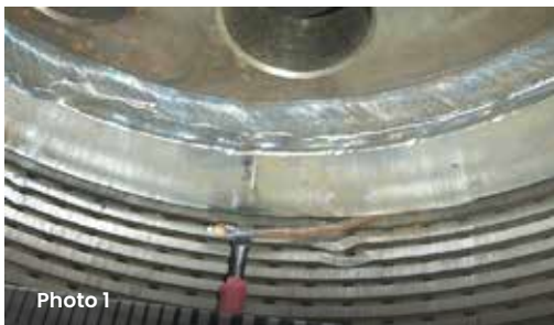
Photo 1 shows weld rod jammed into the trim while photo 2 shows severe gouging of the trim.
