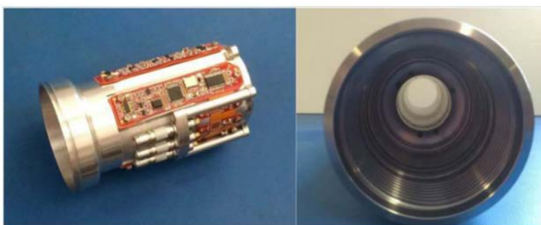
Figure 4—TCT annular ring(left) and module housing(right)(from Garner et.al.2016)
