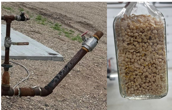
Batch pot on the well head to deliver the pelletized FORSA paraffin inhibitor
