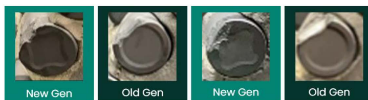
Figure 27—Mixed cutter test results of the new generation general purpose PDC cutter showing reduced material loss.
