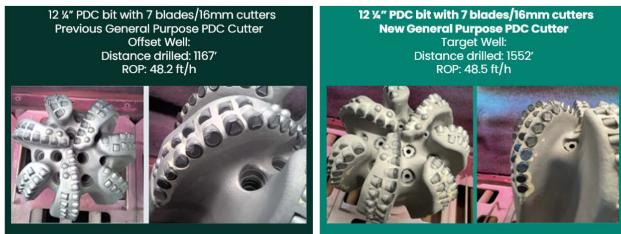
Figure 31—Representative performance and dull photos of 12.25" Haynesville intermediate runs with new generation general purpose PDC cutters compared to offset.
