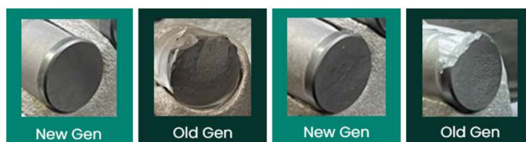
Figure 22—Mixed cutter results of new generation abrasion PDC cutter showing improved durability.
