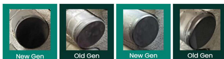
Figure 21—Mixed cutter results of new generation abrasion PDC cutter showing improved abrasion resistance.
