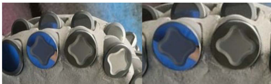
Figure 17—Comparative field test showing strength increase with new multi-dimensional non-planar cutter geometry.
