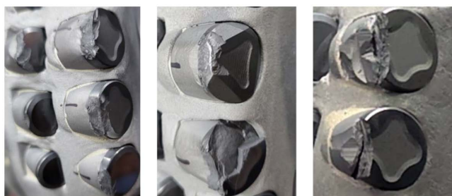
Figure 2—Example dulls of Haynesville intermediate runs.
